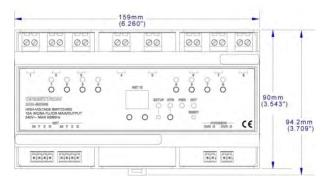
The DIN-8SW8 is an 8-channel high voltage lighting control module designed to support switching of non-dimmable lighting and fans. A single model supports both 120 and 220-240 volt applications. Each channel handles incandescent loads up to 10 amps, fluorescent loads up to 5 amps, and also 1/2 HP motors.
